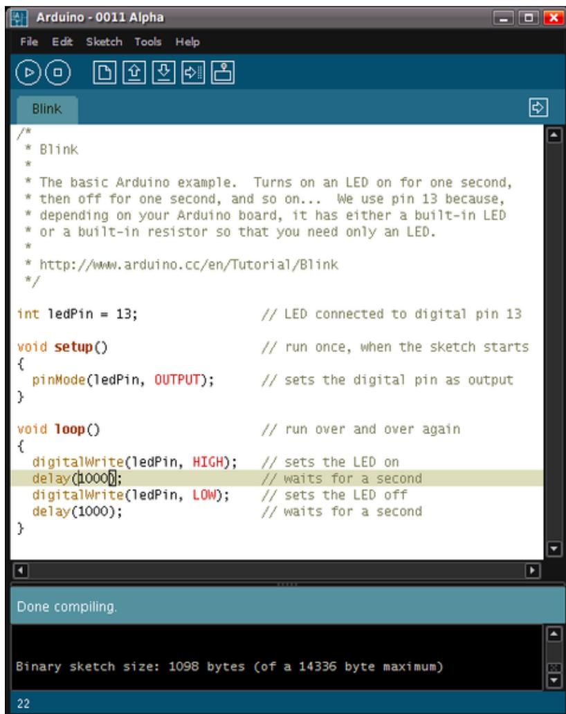
The image shows the Arduino IDE interface. The title bar reads "Arduino - 0011 Alpha". The menu bar includes "File", "Edit", "Sketch", "Tools", and "Help". The toolbar contains icons for running, stopping, saving, opening, and other functions. The main text area displays the "Blink" sketch code. The code is as follows:
